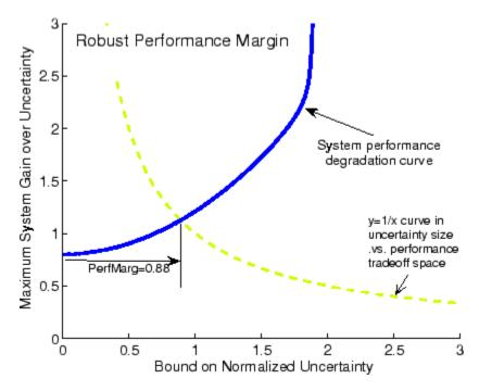
The point where the system performance degradation curve crosses the green line is used as a scalar measure of the robustness of a system to uncertainty. The horizontal coordinate of the crossing point is the *robust performance margin*, PerfMarg.
