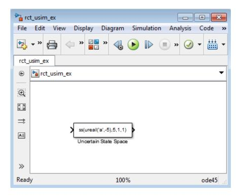
2 In the Simulink model, double-click the Uncertain State Space block to open the Function Block Parameters: Uncertain State Space dialog box, as shown in the following figure.
