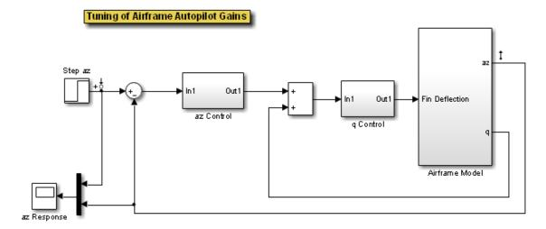
**2** Define a margin analysis point at the output of the Airframe Model block.
